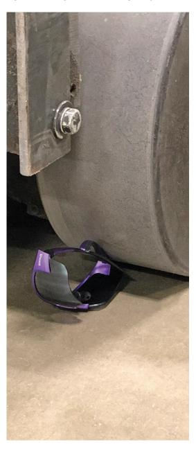
Hercules® is our most durable eyewear line. It passes all the tests established by the American National Standards Institute (ANSI). Additionally, it passes the Global Vision® internal test of the crushing force from our forklift.
